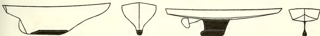
Two types of keels—the full keel ( left ) and the fin type ( right )
